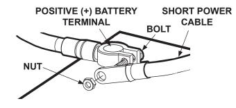
**CONNECTING POWER TO LIFT (TYPICAL)** FIG. 37-1
